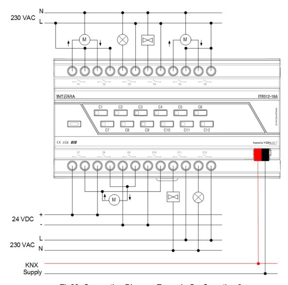
Fig23. Connection Diagram Example Configuration 3
