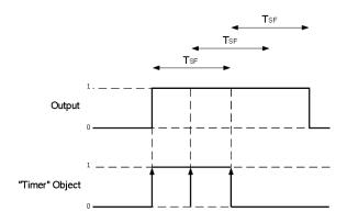
Fig3. Staircase Function Retriggerable
