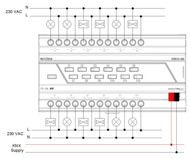
Fig21. Connection Diagram Example Configuration 1
