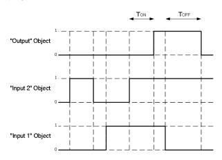
Fig1. Logic Gate with delays
