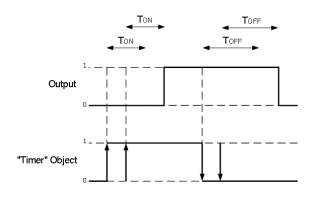
Fig5. ON/OFF Delays Retriggerable
