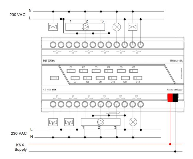
Fig22. Connection Diagram Example Configuration 2
