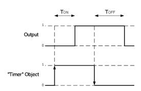
Fig4. ON/OFF Delays
